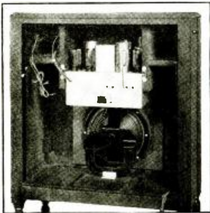
Arrangement of parts (rear view) in the new Radiola battery-operated 8-tube superheterodyne.
